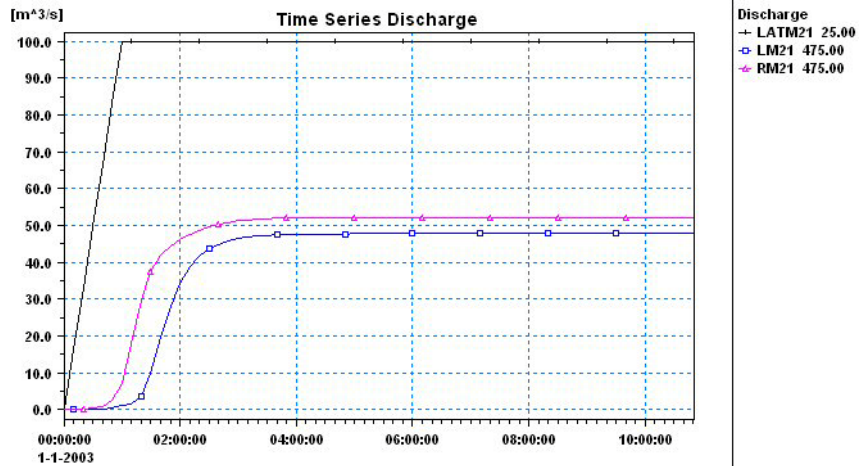
Figure 9.9 Lateral Link Test 1 Results -Time Series of Discharge
