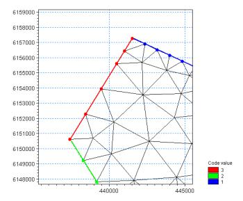
Note the label with the code values. Also note how the node code values extend to the two faces that have nodes with different code values: The land code value is extended to the first node with code value 3 due to the first rule, and the code value 2 is extended to the last node with code value 3 due to the second rule.
