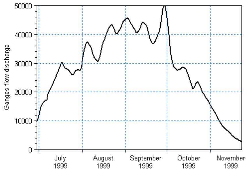
Figure 3.2 Rated flow discharge applied at the upstream Ganges boundary for the 1999 monsoon
