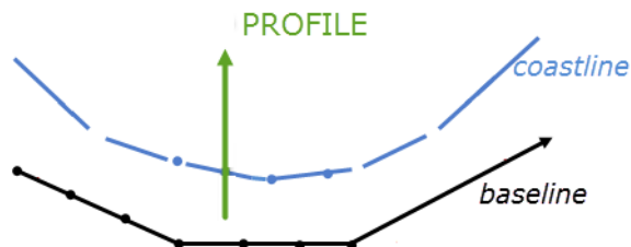
Figure 8.7 Sketch of profile alignment with respect to coastline and baseline
