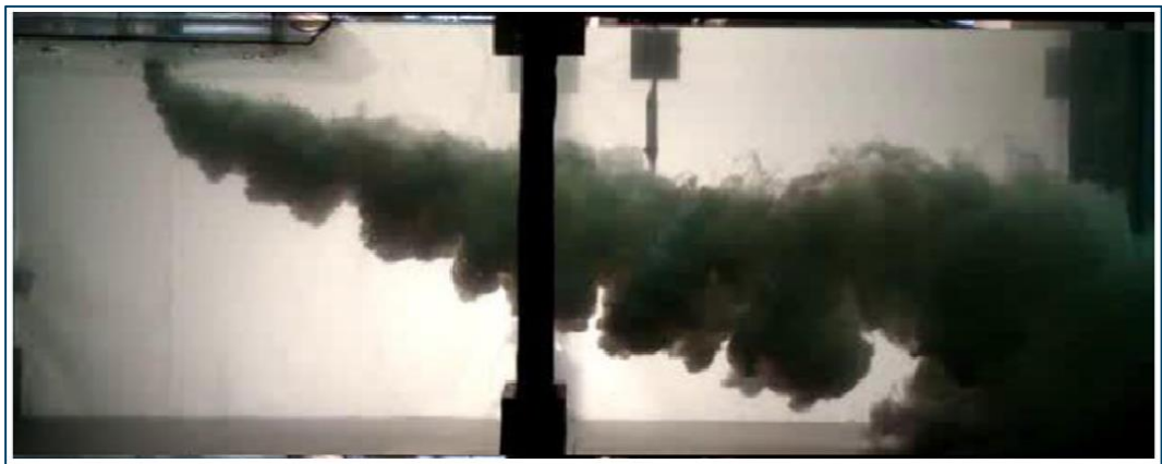
Figure 6.10 Image of the negatively buoyant sediment plume in cross flow (Decrop, 2013)
