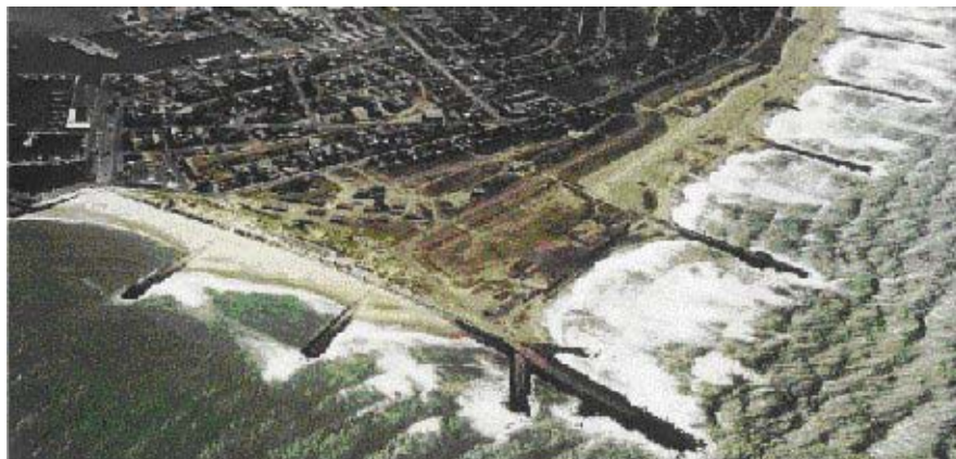
Figure 2.1 MIKE 21 PMS is often used for calculation of wave fields in coastal areas where structures like groynes and detached breakwaters are present
