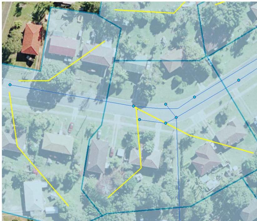
Figure 13.31 Example where two slope lines are drawn from the loadpoint in the network up into the catchment along the normal flow path
