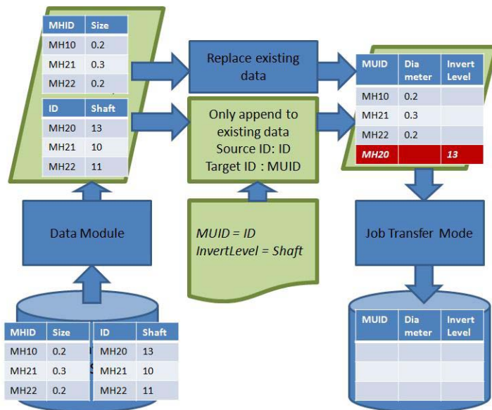
Figure 7.19 Converting the second table to target memory data structure using “Only append to existing data”
