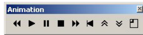
Figure 6.86 Animation allows you to animate the results in time or to select a different time step in which to display results
