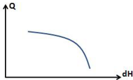
Figure 3.23 Typical example of pump curve
